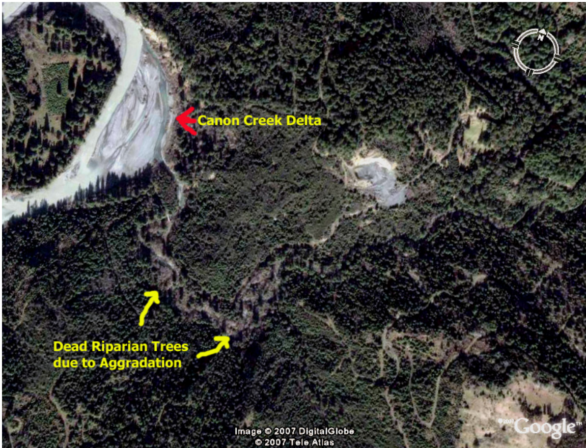
Figure 6. The landscape of lower Canon Creek shows recent timber harvest and an extensive road network. Sediment avulsed from the creek formed a delta at the convergence with the Mad River (upper left) and aggradation in lower reaches of the creek killed riparian trees. Image from Google Earth.
